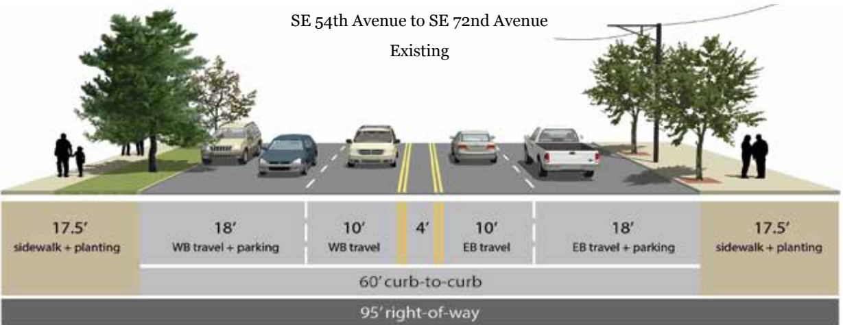
Figure 2-5 Existing and Proposed Cross Sections
