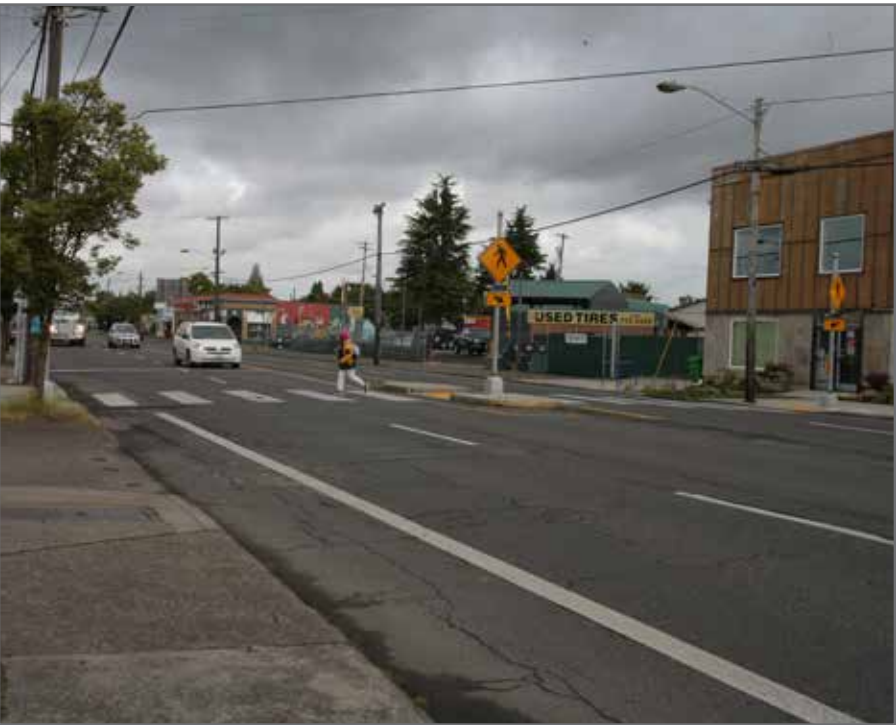
New rectangular rapid flashing beacons (RRFB) improve safety and comfort for people crossing Foster Road.
