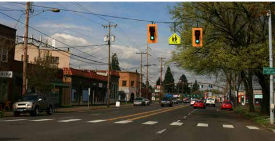
Foster Road has a typical four lane cross section with two travel lanes in each direction, on-street parking and commercial mixed use zoning in the Heart of Foster.
