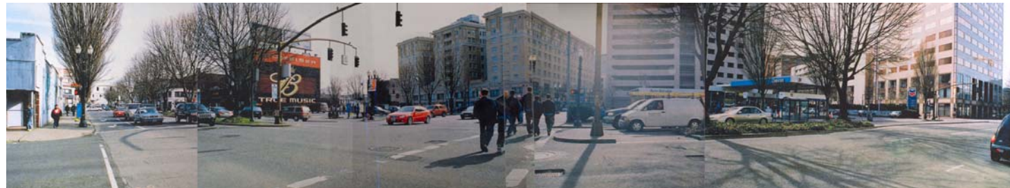
Long pedestrian crossings, narrow sidewalks, lack of left turns and no on-street parking contribute to the "Burnside barrier". This view is of Burnside looking southeast from NE 4 th Avenue.
