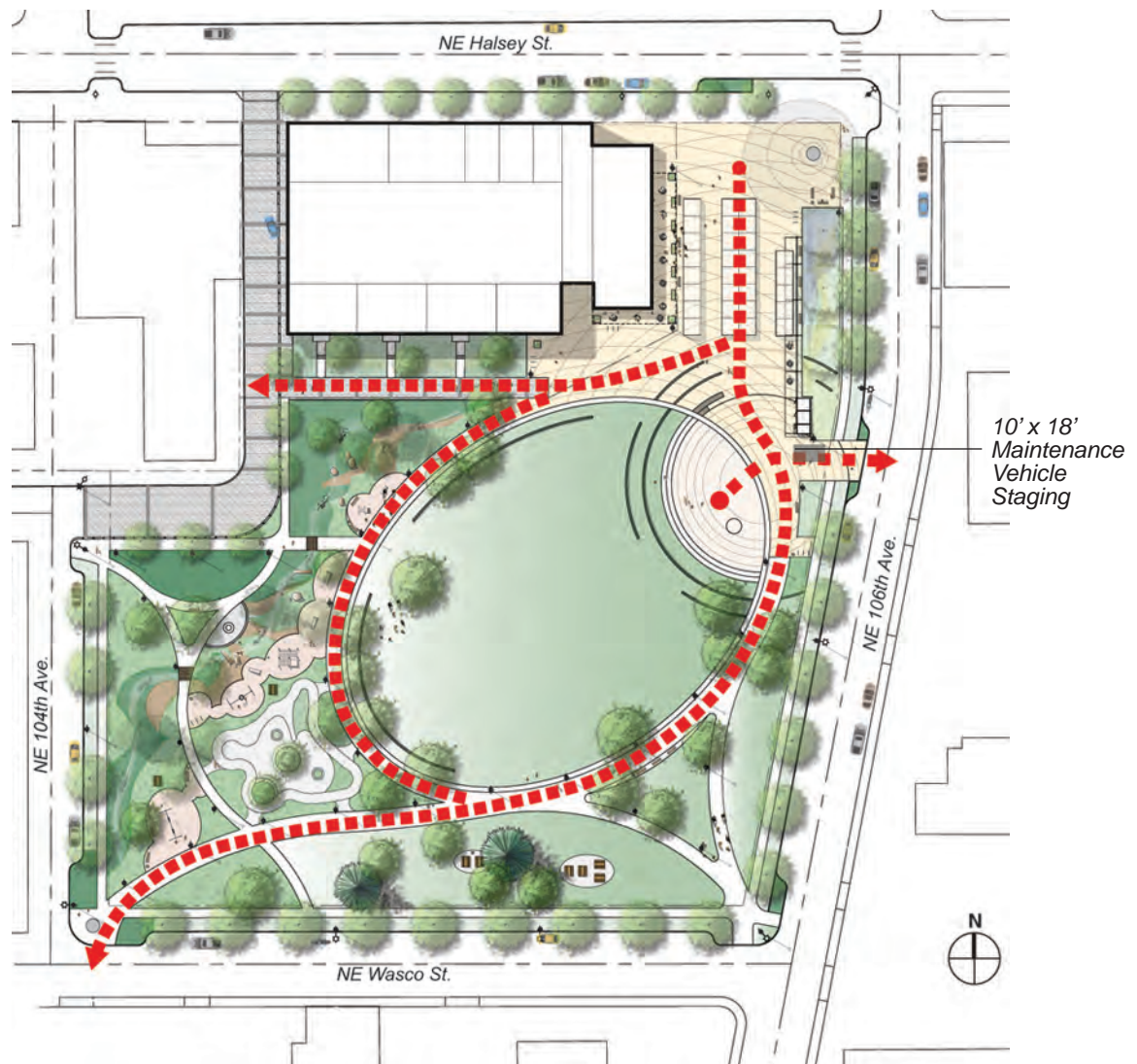
Maintenance and vehicular access shown in red.
